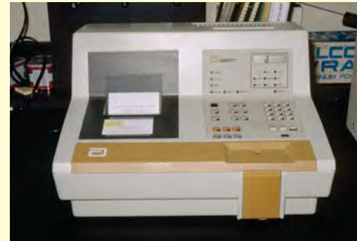
ABOVE Figure 4.7 The self-contained instrument provided for reading the Chlamydiazyme EIA assay.
